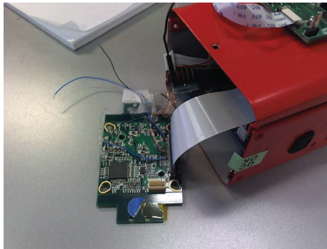
Figure 10. Appro IP Camera with IMX172 and MachXO2 with SubLVDS to CSI-2 Bridge
