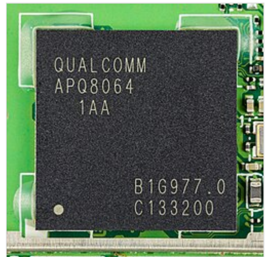
The APQ-series SoC does not feature an on-chip cellular modem. This APQ8064, for example, requires an external modem; it was marketed as the Snapdragon 600 .
