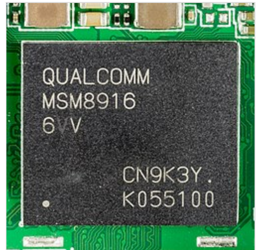
A surface-mount MSM8916 on a printed circuit board (PCB), showing the outer surface of its plastic packaging , with laser-engraved model numbers . This SoC is marketed as the Snapdragon 410 .
