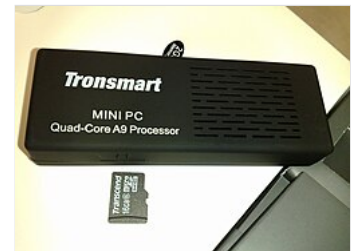
Tronsmart MK908, a Rockchip-based quad-core Android "mini PC", with a microSD card next to it for a size comparison.
